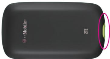
2. Remove the battery and mylar strip protecting the battery compartment. Slide the SIM card into the SIM card slot, as shown and write down the default SSID and password printed on the label in the battery compartment.
