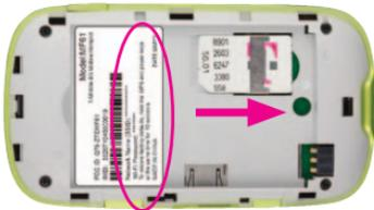
3. Align the metal contacts on the battery with the metal contacts in the battery compartment and press the battery into place. Replace the battery cover.
