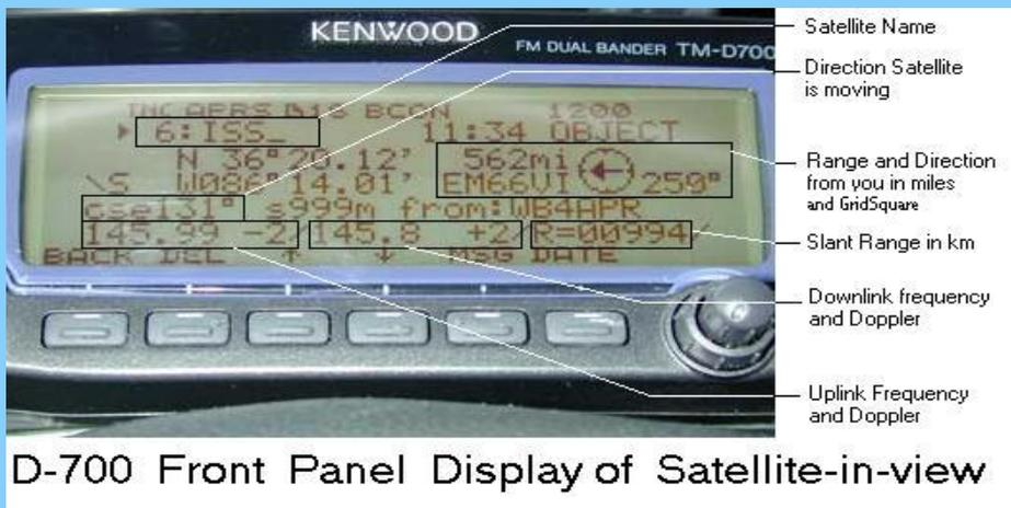
D-700 Front Panel Display of Satellite-in-view
