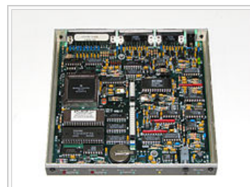
The Kantronics 9612+ was implemented around an 8-bit Motorola microcontroller.
